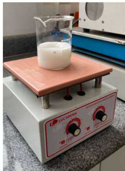
Figure 4. Nitric acid, aluminum hydroxide, and water being homogenized by magnetic stirring, from authors (2025)
