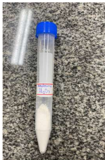
Figure 6. Alumina nanoparticle production completed, from authors (2025)
