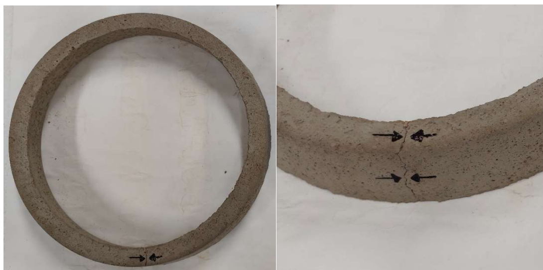
Figura 55: Anel de argamassa com RCV 1,0:6,0:1,12.
