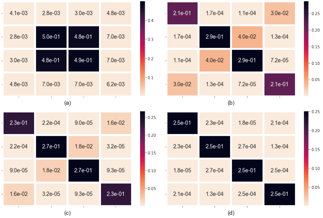
Figure 4 – Thermal states obtained in the simulation for different temperature values: (a) thermal state at T = 5 \times 10^{-4} K ; (b) T = 10 K ; (c) T = 20 K ; (d) T = 300 K . All these thermal states were reproduced after 400 simulation steps, with J/k_B = 1 K , where J and k_B are the magnetic coupling and the Boltzmann constant, respectively.
